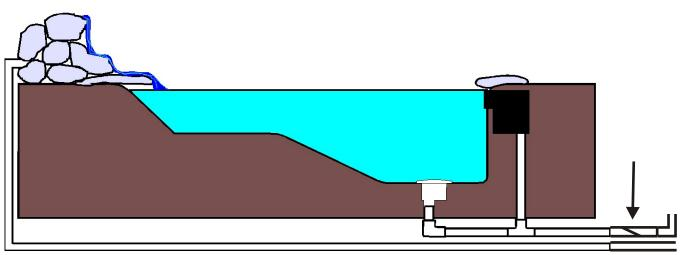
Swing check valve installed below water level in an easily accessed location will make keeping the pump and Turbovortex primed much more easy.
