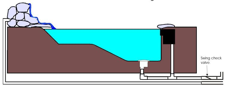
Swing check valve installed below water level in an easily accessed location will make keeping the pump and Turbovortex primed much more easy.
