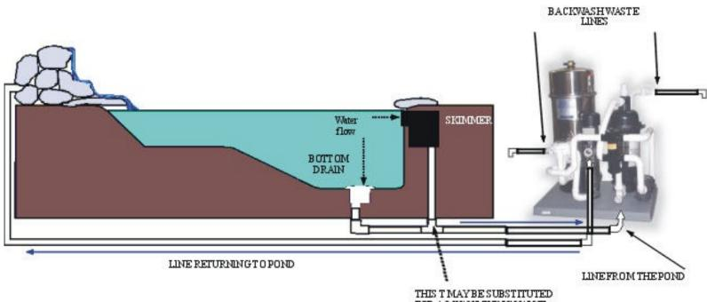
THIS T MAY BE SUBSTITUTED FOR A 3 WAY MIXING VALVE AND MOVED CLOSER TO THE EQUIPMENT PAD. THIS WILL ENABLE YOUT O VARY THE AMOUNT OF FLOW COMING FROM THE BOTTOM DRAIN AND SKIMMER.
